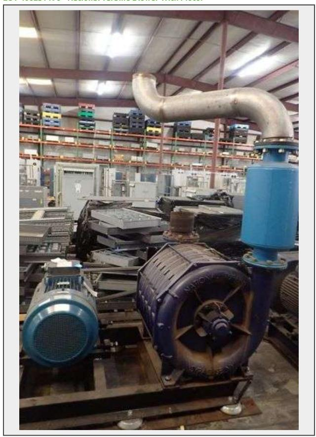
(1) National Turbine Blower With Motor, Cat No. MT55306-3-3-AD, Includes; (1) ABB Motor, Cat No. MBT-225-m-4, 3PH, 660V, 50A, 60HP; Tag: 309240 | Location: 2-G
