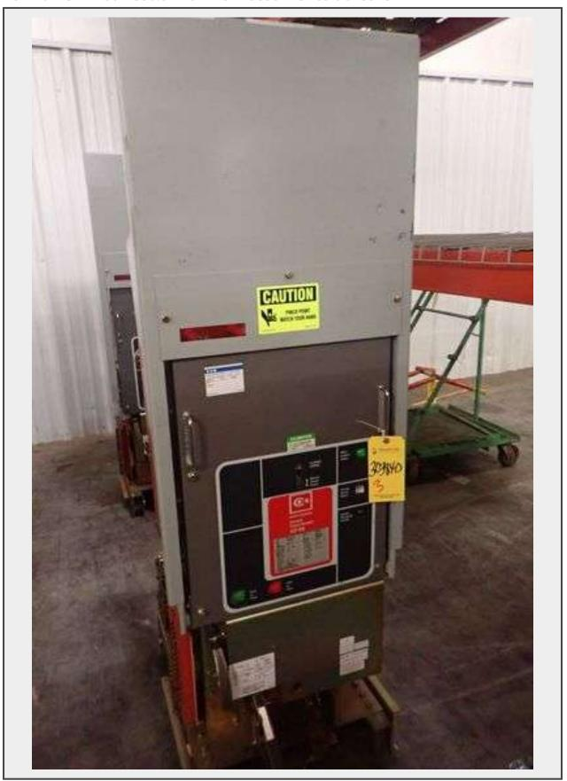
VCP-WR, Rated Max Volts: 4.76 KV, Rated Cont Current: 1200A, Motor Volts: 125 VDC, Close Current: 6.6 A, Voltage Range: 90-140 VDC, Breaker Operation Counter: 534, 700 lbs; Tag: 303840 | Location: 5-D
